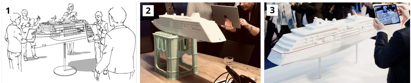
Figure 5: Evolution of an application featuring a physical model in a handheld application on iPads: From (1) sketch over (2) substitution prop to the (3) final physical model (P12).
