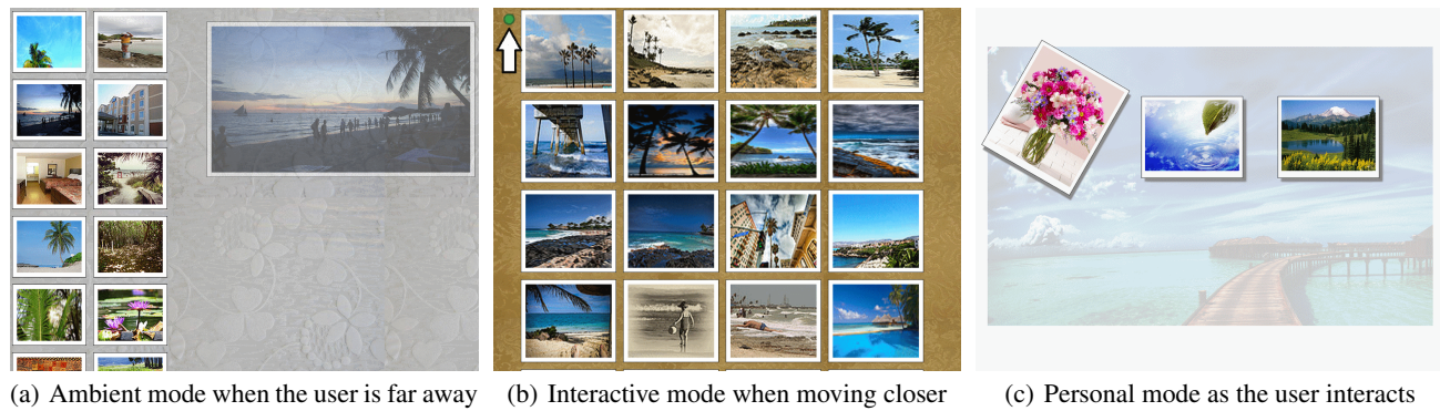
Figure 5. Fotobook application using XDKinect with support for hand-as-cursor interaction and different interaction zones
