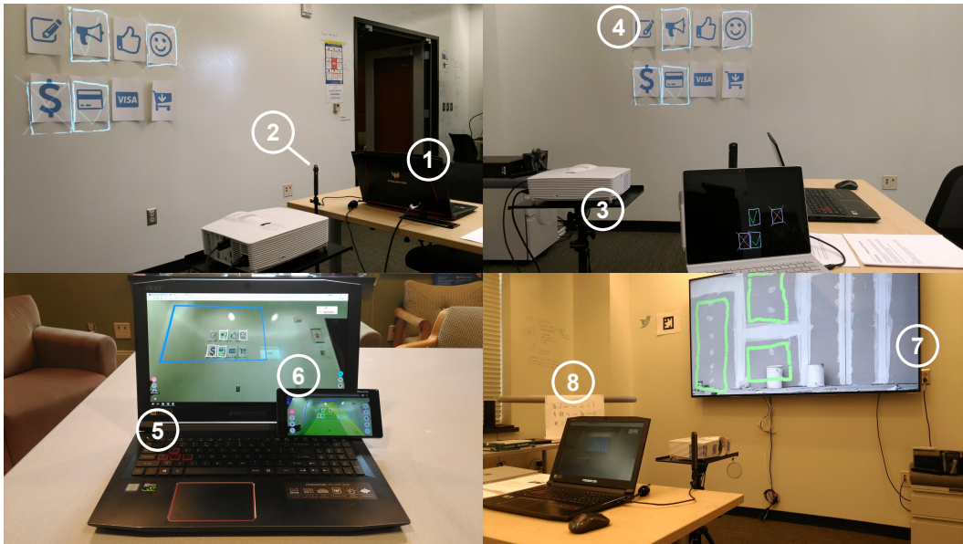
Fig. 5. The design jam set-up: (1) an Acer Predator Notebook connected to (2) a RICOH Theta S 360-degree camera for the local participants; (3) a projector connected to a Microsoft SurfaceBook; (4) icons provided for scenario #1; (5) another Acer Predator Notebook for one remote collaborator; (6) an ASUS ZenFone AR for the other remote collaborator; (7) a 4K screen acting as the second projection in scenario #3; and (8) hieroglyphic symbols for scenario #2.
