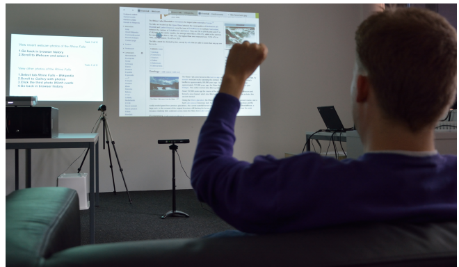
Figure 2. Study setup consisting of a Kinect and a large screen for Kinect Browser, as well as a camera for video recording.
